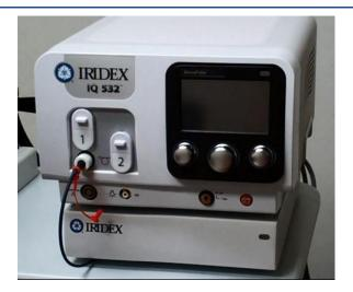
10. Carefully route the fiber optic cable under the control box making sure the feet of the control box do not rest on the cable and the cable is unconstrained. Connect fiber to the front of the laser console into either port 1 or port 2.
